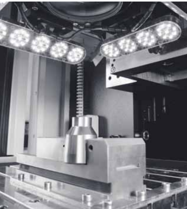
Machine workspace with marking head, IMP lighting, and component. Examined and tested in more than one hundred installations, IMP detects the position of parts and components and automatically and precisely specifies the geometry data that is required for laser marking and engraving.
