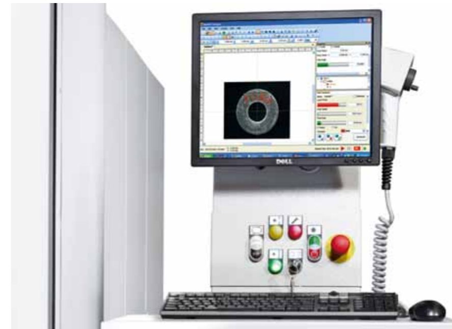
Point & Shoot™ application on a flat washer, camera view in the FOBA MarkUS™ operating interface
